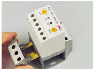
② Cable connection part can be modified between screw connection and passing CT hole
